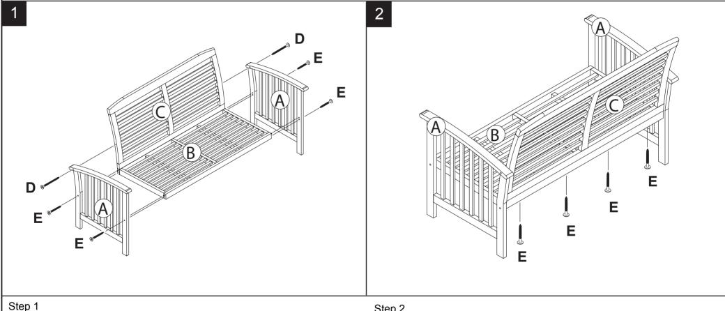
Attach leg frame (A) to back frame (C) ,use screws-1 (D),tighten with allen key(H1).Use screw -1 (E) to connect leg frame (A) with seat frame (B), tighten with allen key (H1).
